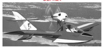
The Osprey is a 2-place amphibian aircraft with fully retractable landing gear. The Osprey utilizes wood and steel construction and is ideal for the first time builder seeking well presented plans, ease of construction, and the versatility of an amphibian aircraft.
