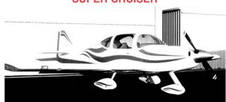
The Super Cruiser is a 4-place aircraft with a cruise speed of 190 mph and a stall speed of 59 mph. The aircraft has a length of 25.46 ft. and wing span of 29 ft. It has a gross weight of 2500 lbs. and a useful load of 1100 lbs. The prototype is powered by a Cont. IO-360ES. Lycoming engines from 160-200 HP are recommended and build time is 1200-1500 hours. Aircraft Spruce is a prime supplier for materials used in Super Cruiser kits.
