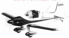
The Corby Starlet is an all wood single seat, low wing cantilever monoplane. It is a very practical cross-country machine as well as being an aerobatic aircraft. The design was drawn around the use of VW powerplants up to 75 hp and 160 lbs. max. The Starlet has been awarded a Type certificate issued by the Australian Aviation Authority. For more info contact:
