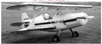
Design lines out of the past with the performance of today. With a 64 hp VW engine the Easy Eagle cruises at 100mph and has a stall speed of 45mph. The Easy Eagle features a fabric covered fully welded steel frame combined with an all wood wing. It has a one piece landing gear and fully steerable tail wheel for easy ground handling. Takeoff run and landing roll are both approxl 300ft. Aircraft Spruce supplies full materials kits for Easy Eagle. Contact us for free kit list.
