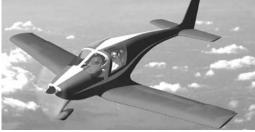
The Nexaer LS1, a 2-seat composite airplane that meets Light Sport Aircraft classifications under the new FAA Sport Pilot rule and is being promoted and marketed by Sportplanes.com The LS1, manufactured by Nexaer in Colorado Springs, Colorado, fetures a 54" wide cockpit, a cruise speed of 120 knots and a useful load in excess of 600 lbs. The prototype of the LS1 was unveiled at AirVenture 2005.
