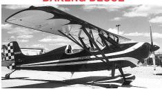
The Bakeng Deuce is a two place parasol that is great for plain every day or weekend flying. It is of a basic aircraft design utilizing a steel tube fuselage. The structure is faired with plywood and aluminum formers which support spruce stingers. Wings are of basic wooden construction with solid spruce spars. The Deuce is a very easy aircraft to build with an excellent set of plans. It has a max. speed of 140 mph, cruises at 110-120 mph with a stall speed of 35-40 mph.
