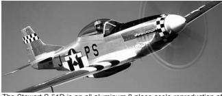
The Stewart S-51D is an all aluminum 2-place scale reproduction of the North American S-51D Mustang. The aircraft features dual controls and is fully aerobatic. The S-51D utilizes liquid colled engines ranging from 300 to 700 hp. The 91" diameter, constant speed fourblade Hartzell propeller is driven through spur gear reduction with a 0.469 (2.13:1) ratio. Using a 400 hp engine, the S-51D duplicates S-51 performance, except for top speed.
