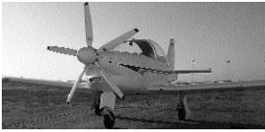
The Alfa is a European kit built aircraft. The Alfa is an all-metal low-wing. tri-cycle gear airplane with side-by-side seating. The aircraft is 19.35ft in length and has a wing span of 29.5 ft. Suggested engine for the plane is a 110 HP Volkswagen Porsche G 2 2.400 air cooled boxer engine. The HB207 cruises at 140 kts with an fuel burn of 3.5 US Gal/hr and stalls (flaps down) at 40 kts. It features a 5 blade constant speed prop, retractable landing gear, and detachable wings.
